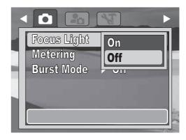
4 Press ▲ or ▼ to highlight On or Off, then press SET to save and apply the setting. The focus assist light icon appears on the LCD monitor.
