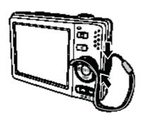
2 Thread the larger loop of the strap though the short loop, then pull the strap tight.
