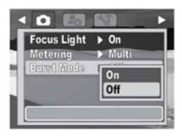
4 Press ▲ or ▼ to highlight On or Off, then press SET to save and apply the setting. The burst mode icon appears on the LCD monitor.
